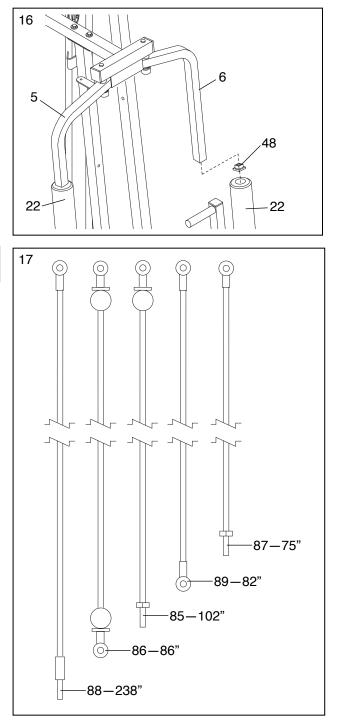
Insert a 5/16" x 1" Bolt (95) through the bracket on the Right Butterfly Arm (5). Tighten a 5/16" Nylon Jam Nut (91) onto the Bolt.
